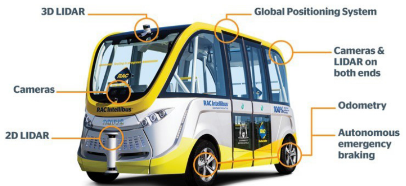
Figure 1.1 Navya sensor platform Image source: curbsideclassic.com
